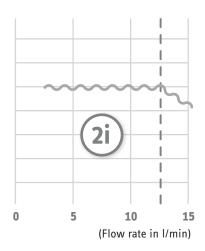
Practically constant DHW temperature up to the output limit, then decreasing at higher flow rates
