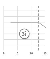
Constant DHW temperature up to the output limit, then decreasing at higher flow rates
