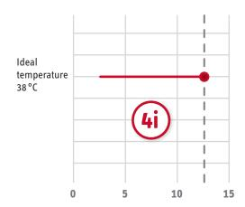
Constant DHW temperature at all times. When the output limit is reached, the flow rate is maintained fully automatically with the maximum water volume.
